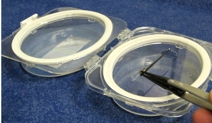
Figure 3-20: Inserting the Stylus Tip into the Hole in the Film in the Stylus Case
